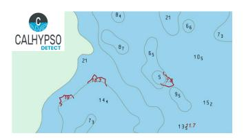
CALHYPSO-Detect dangers detection tool compare a new survey dataset with active ENC maps on this region and highlight unmapped dangers. These detections can be broadcart as notices to mariners. The amount of detections raised during this first analysis can also justify the production on a new map on this region.
