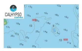
CALHYPSO-Control generalisation control tool looks for cartographic representation errors in a S-57 ENC. The algorithm alert on anomalies related to security risks and on representation deviations from readibility rules required. To this end, the tool compare a produced ENC with its source survey dataset.
